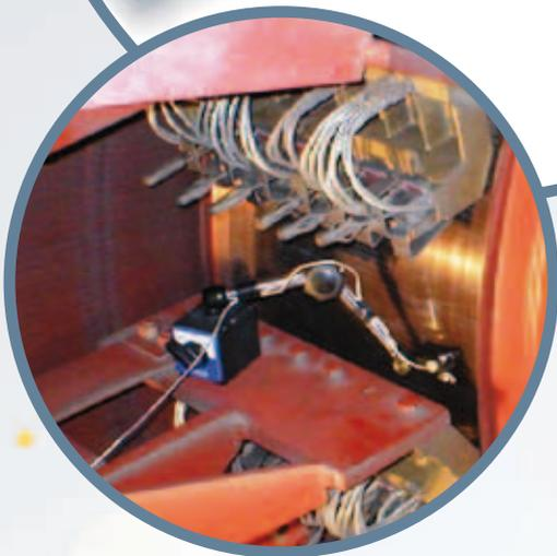
The new ComPro2000™ distributed by Mersen is a portable diagnostic tool to quickly and easily determine the health of your motor's commutator.
